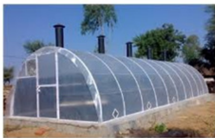
Dome shape dryer with chute vents
