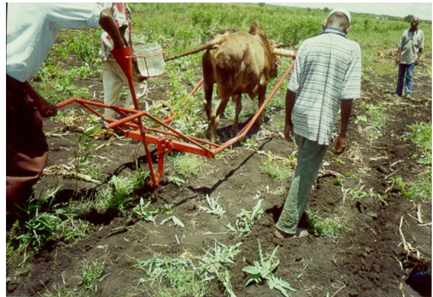
Dry planting tool with tubes for seed and fertiliser
